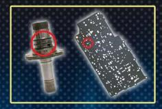
JASPER offers upgrades to the early-style GM 6L80/90 transmission such as a modified stator support shaft with updated 1-2-3-4 and 3-5/reverse seal rings and a notched valve body spacer plate gasket.
