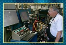
**Every JASPER Transmission undergoes** dynamometer testing to ensure proper gear ratios, line pressure, cooler pressure, cooler flow, and quiet operation. The TCM, on the GM 6L80/90, is validated using a state-ofthe-art CAN software package.
