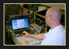
The TEHCM for the GM 6L80/90 is 100% tested with JASPER-designed test equipment to verify communication between the computer and all internal inputs including: transmission fluid pressure switches, temperature sensor, speed sensors, internal mode switch, and solenoids.
